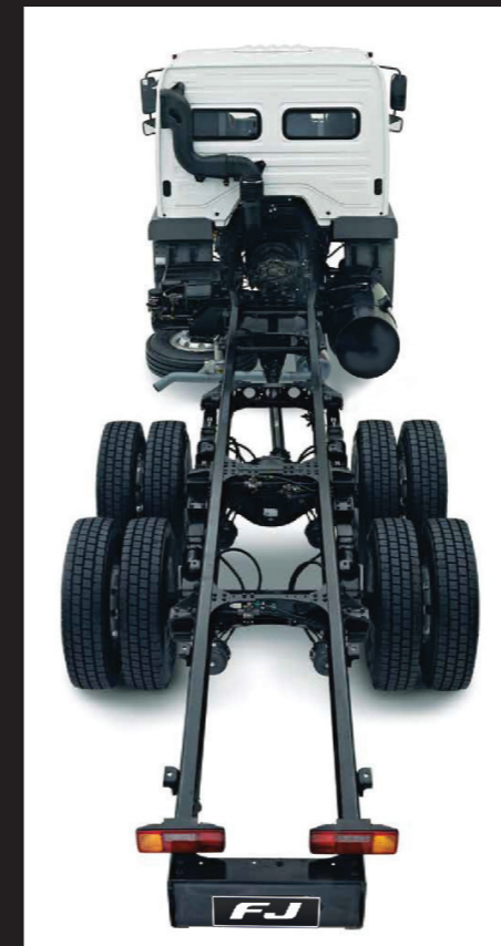
The frame is shot-peened and powder coated to prevent corrosion and increase durability. Higher flange width and web height also offer stability and load bearing ability leading to longer frame life while the alligator type cross members make it exceptionally strong.
