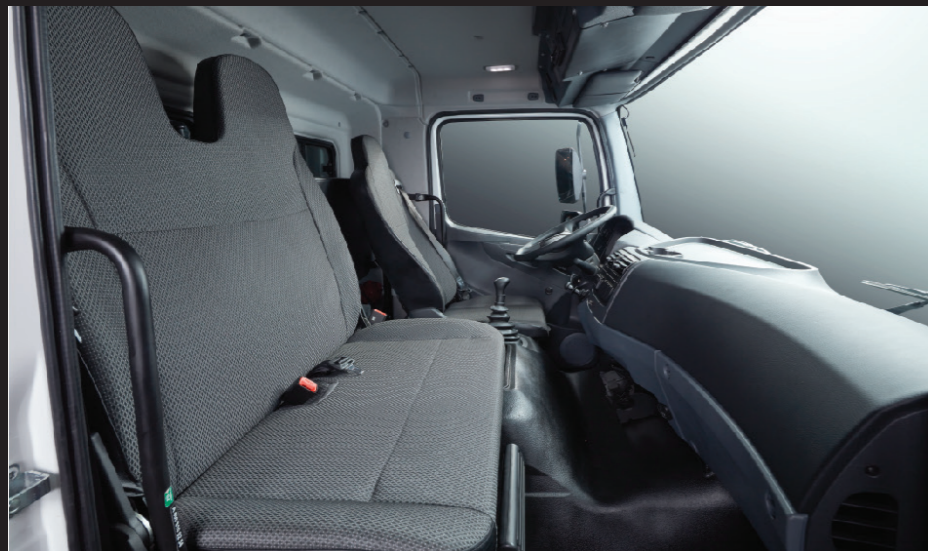
The multi-adjustable air pressure driver's seat and tilt and telescopic adjustable steering wheel allow the driver to set the optimum driving position for comfort and performance.
