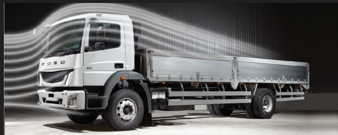
The FJ's aerodynamic cab design reduces wind resistance thus reducing cabin noise while increasing fuel efficiency
