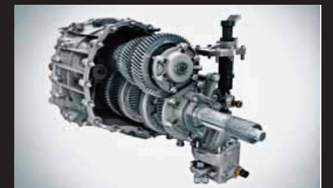
The Fuso FJ is equipped with a smooth-shifting 9-speed manual transmission which provides a higher flexibility of gear selection for various operating conditions thereby enhancing driving performance and improving fuel efficiency
